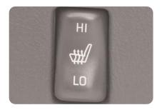
Your vehicle's driver and passenger seats can be heated. The controls are located on the outboard side of the driver and passenger seats. Both the lower cushion and lower seatbacks can be heated. For the low setting, press the lower portion of the switch. For the high setting, press the upper part of the switch. To turn the heat feature off, move the switch to the center position.
